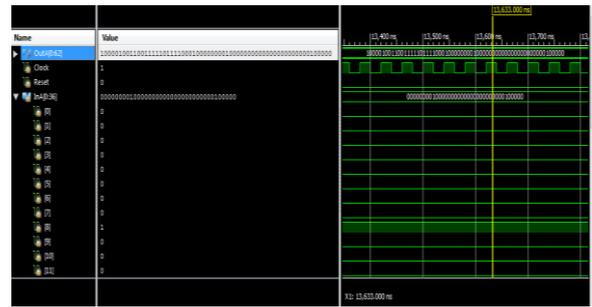
Fig 4.1 Simulation output for Parity check matrix generation
