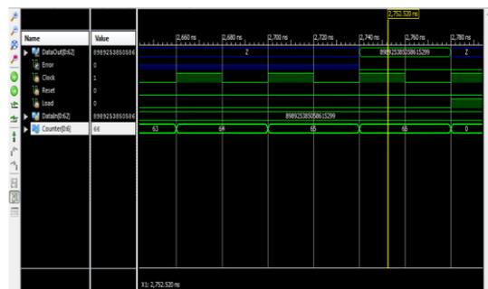
Fig 4.2 Simulation result for decoder output without error
