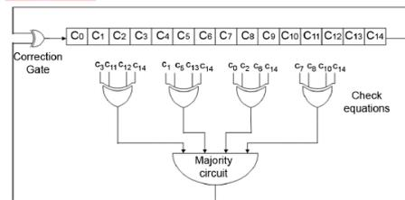
Fig.3.3 Serial one step majority logic decoder for the (15,7) EG-LDPC code
