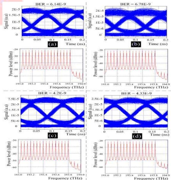
Figure 5. Eye diagrams and spectra at the input (a,c) and at the output (b,d) of the discrete amplifier: of the 9<sup>th</sup> channel of the system with SOA (a,b) and of the 15<sup>th</sup> channel of the system with EDFA (c,d).
