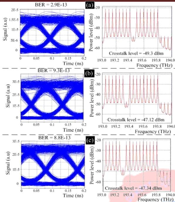
Figure 4. Eye diagram and inter channel crosstalk of the 9<sup>th</sup> channel of the system with the DRA (a), of the 7<sup>th</sup> channel of the system with the hybrid DRA-EDFA amplifier (b), and of the 6<sup>th</sup> channel of the system with the hybrid DRA-SOA amplifier (c).
