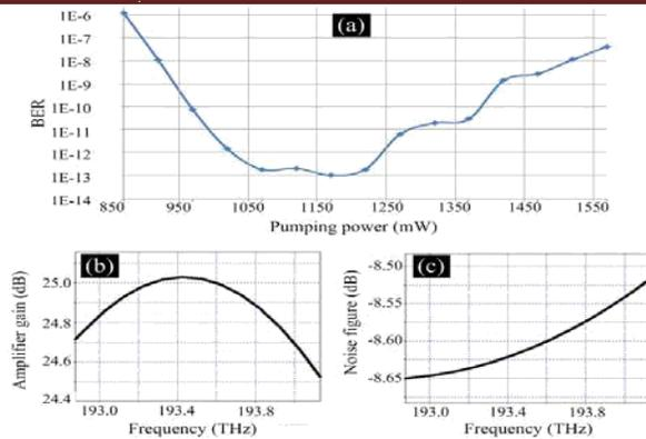
Fig. 2. System BER value dependence on the 1451.8 nm co-propagating pump power (a) of the DRA, and gain spectrum (b) and noise figure (c) of the DRA at 1150 mW pump power.
