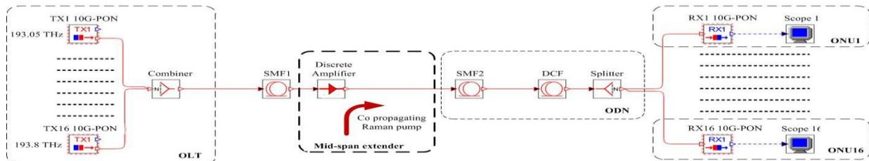
Fig. 1. Simulation scheme of the 10 Gbit/s long reach DWDM optical access system with hybrid DRA-EDFA and DRA-SOA amplification.
