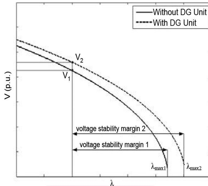
Fig. 2. Impact of a DG unit on maximum loadability and voltage stability margin
