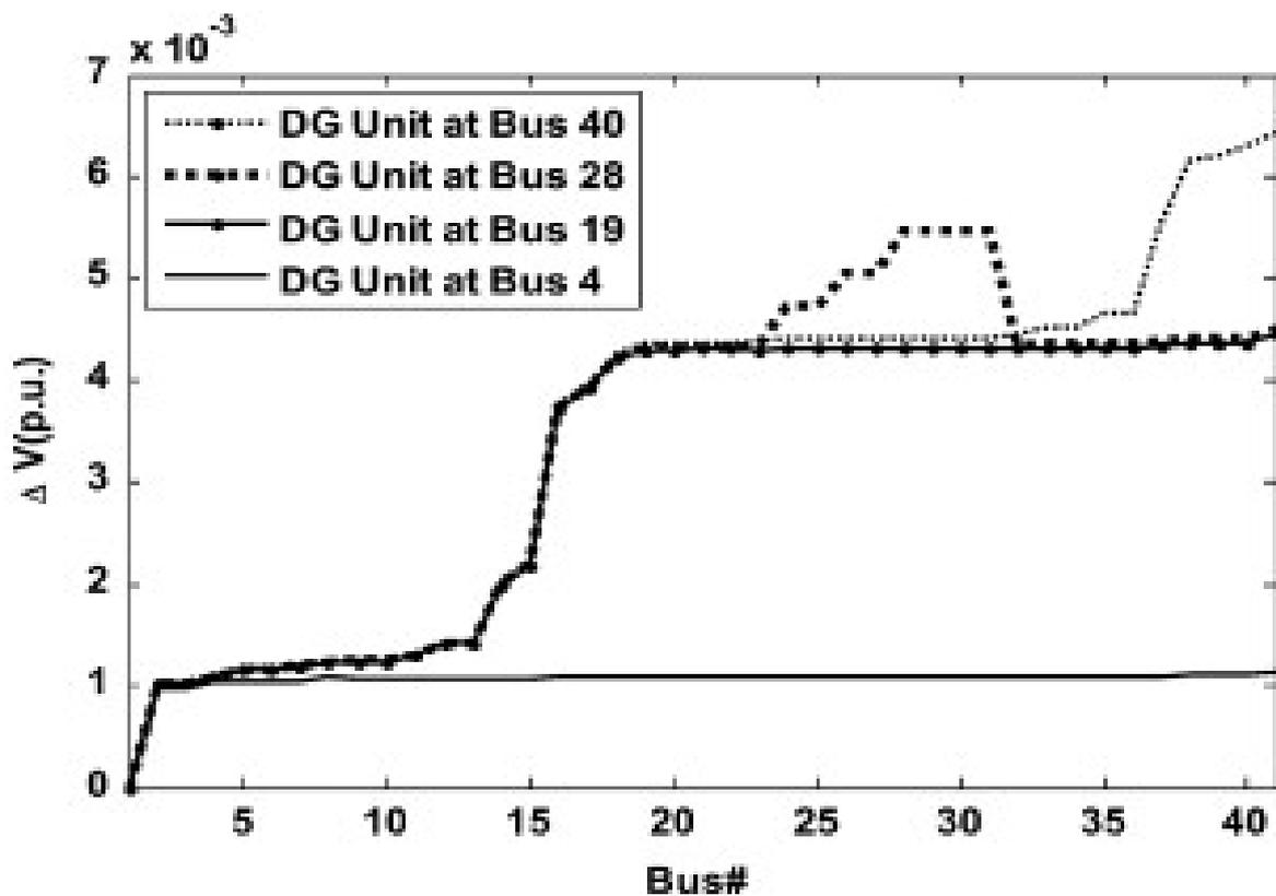
Fig. 6. Results of voltage sensitivity analysis  $\Delta V / \Delta Q$
