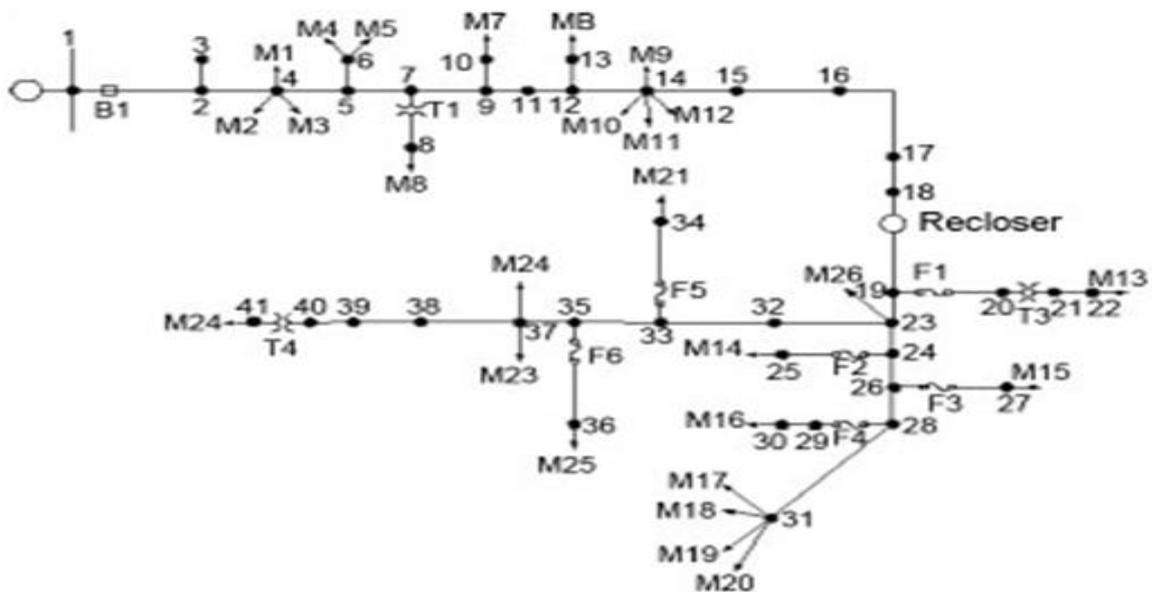
Fig. 3. Sistribution test system of 41 buses
