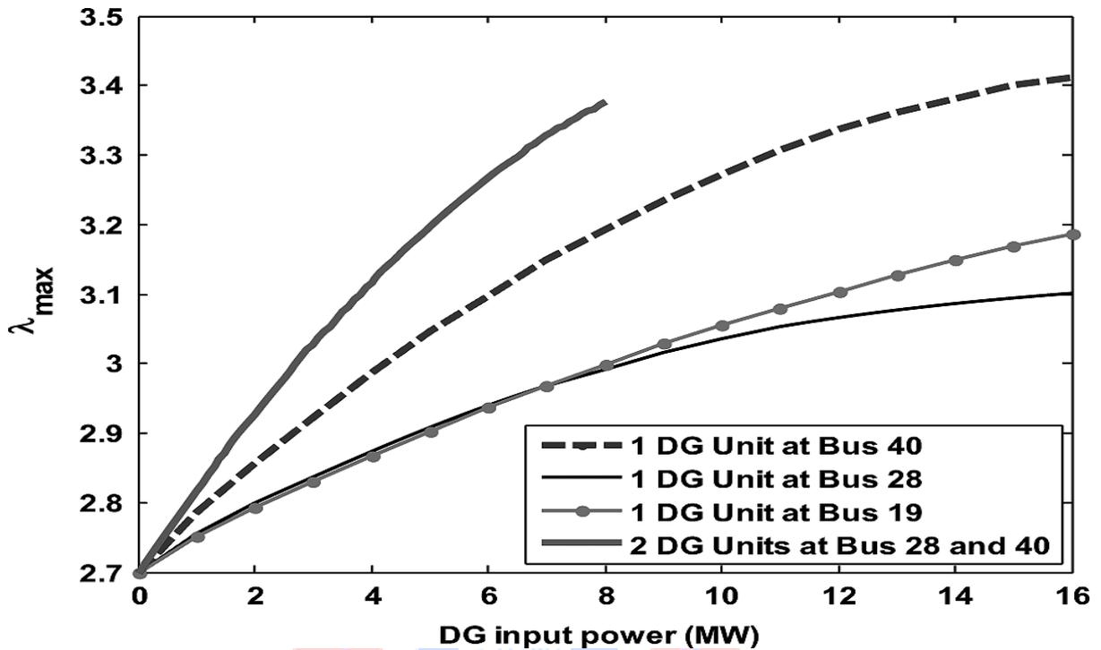
Fig. 5. Impact of the size of the DG units on maximum loading
