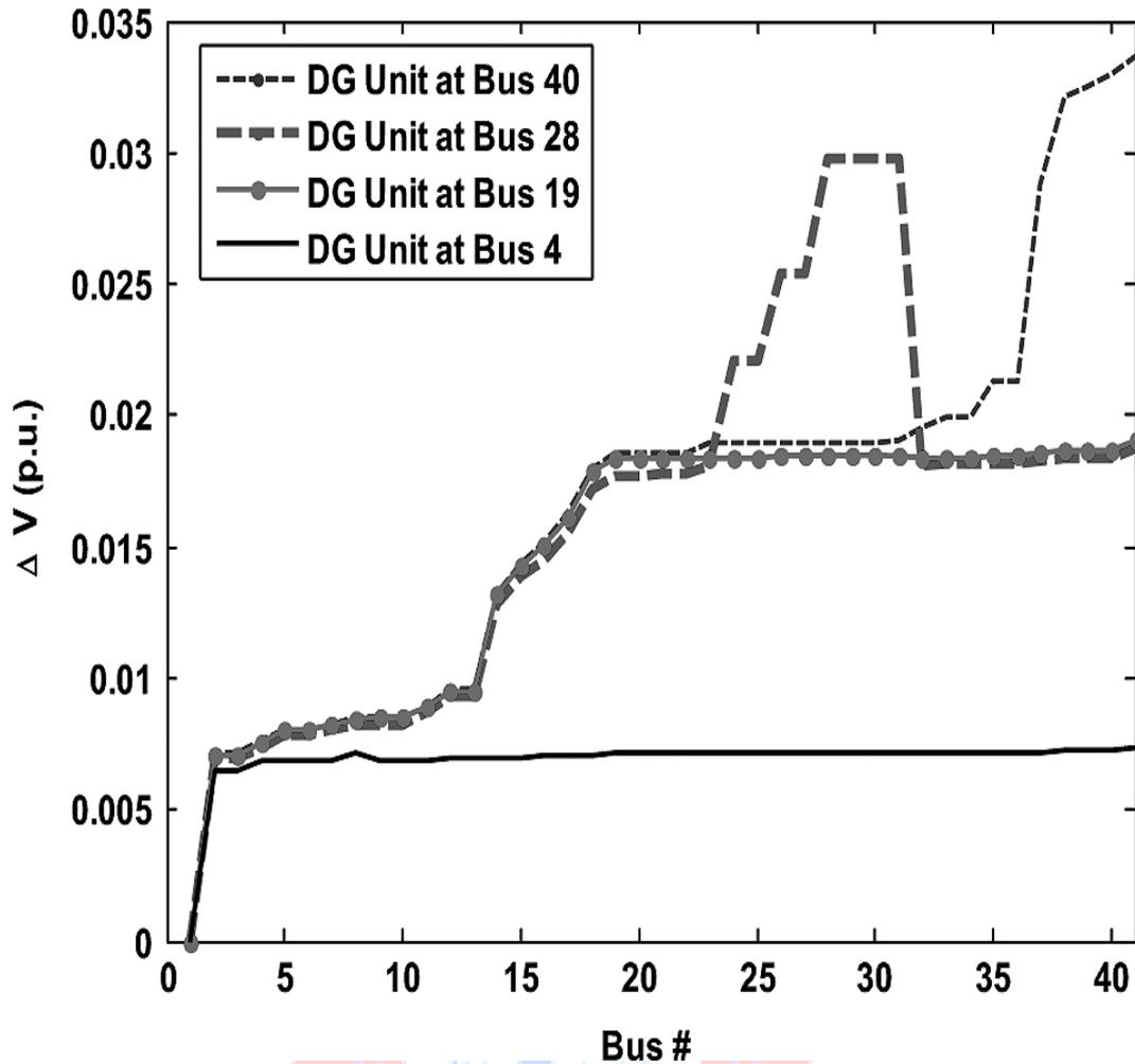
Fig. 4. Results of voltage sensitivity analysis (the penetration level is 30%).
