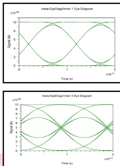
**Fig No : -3.1.3 Received eye diagram for optical effective index equal to 3.0 and electrical effective index equal to 3.0 (top) and 3.4 (bottom)**
