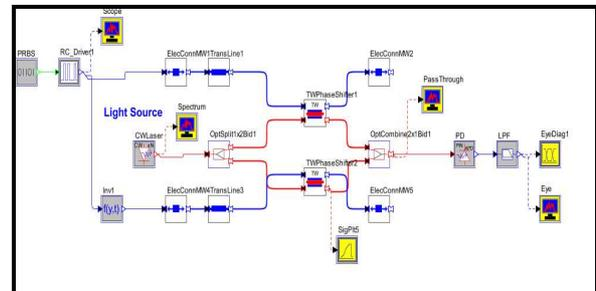
Fig No: - 2.2 Layout of a Traveling Wave Mach-Zehnder modulator PIC with microwave circuit connecting the electrodes to the generator and load impedances
