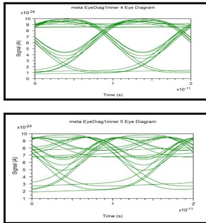
Fig No : - 3.2.2 Eye diagrams at the receiver with traveling wave electrode impedance equal to 50 Ohm and load impedance equal to 40, 30 , 20 and 10 Ohm (from top to bottom in sequence)
