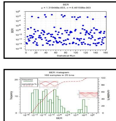
Fig No: -3.3.2 Distribution (top) and histogram (bottom) for the BER at back-to-back received signal
