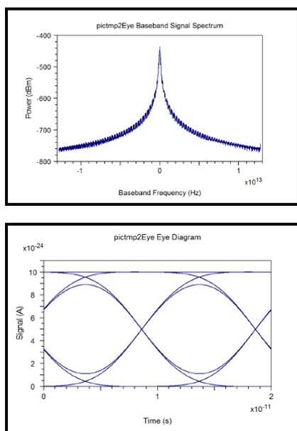
**Fig No : - 3.1.2 Detected signal (top) and receiver eye diagram (bottom)**
