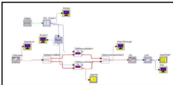
Fig No: - 2.1 Layout of a Traveling Wave Mach-Zehnder modulator PIC
