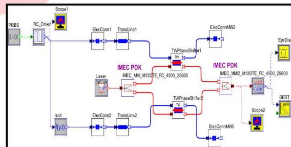
Fig No: - 2.3 Layout of the transmitter chip using TW-MZM.
