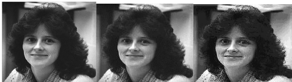
Original Image1(83kb) Compressed Image (5.52kb) Decompressed Image (30.9kb) Figure 11: Compression and Decompression of Image 1
