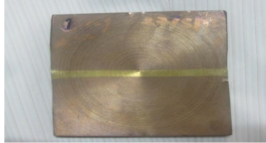
(i) Test Plate one reveals are free from Visual Defects
