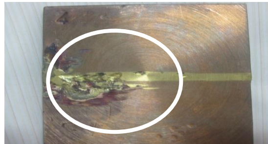
(iii) Test Plate three reveals Shrinkage and Burn Through
