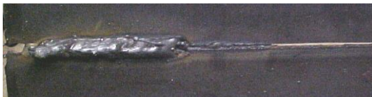
Figure 7: Excessive penetration and / or Reinforcement
