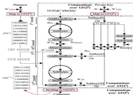
Fig. 4 Proposed masked AES with an unrolled architecture in CBF mode and OFB mode
