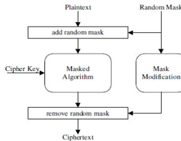
Fig 2.1 Basic Masking Principle
