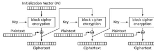
Fig 4.3 Cipher Feedback Mode Encryption
