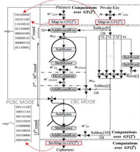
Fig. 4 Proposed masked AES with an unrolled architecture in CBC mode and PCBC mode
