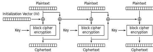
Fig. 4.2 Propagating Cipher block chaining mode encryption [7]
