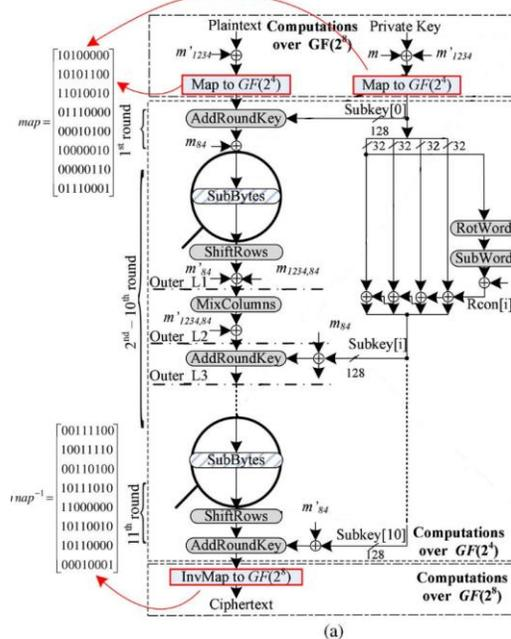
Fig.1 Proposed masked AES with an unrolled architecture of Masked AES with pipelining technique
