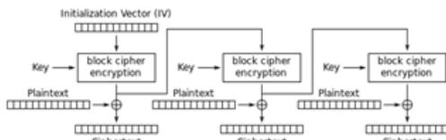
Fig 4.4 Output Feedback Mode Encryption
