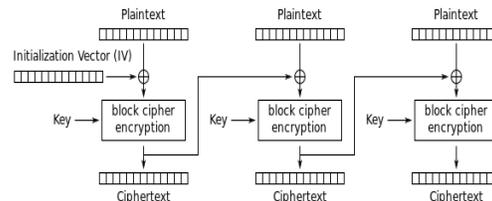
Fig. 4.1 Cipher block chaining mode encryption [7]
