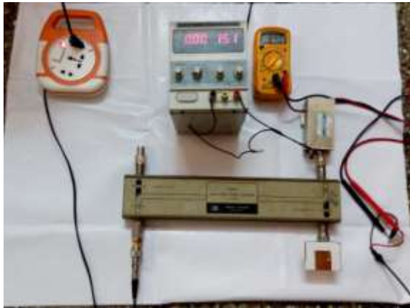
Fig 6:Return loss Measurement setup for single element cloth antenna
