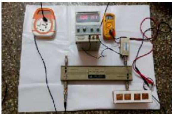
Fig 7: Return loss Measurement setup for four element array cloth antenna
