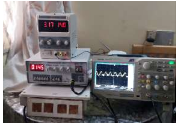
Fig 10:FM-CW test bed with the cloth antenna array visible in the photo
